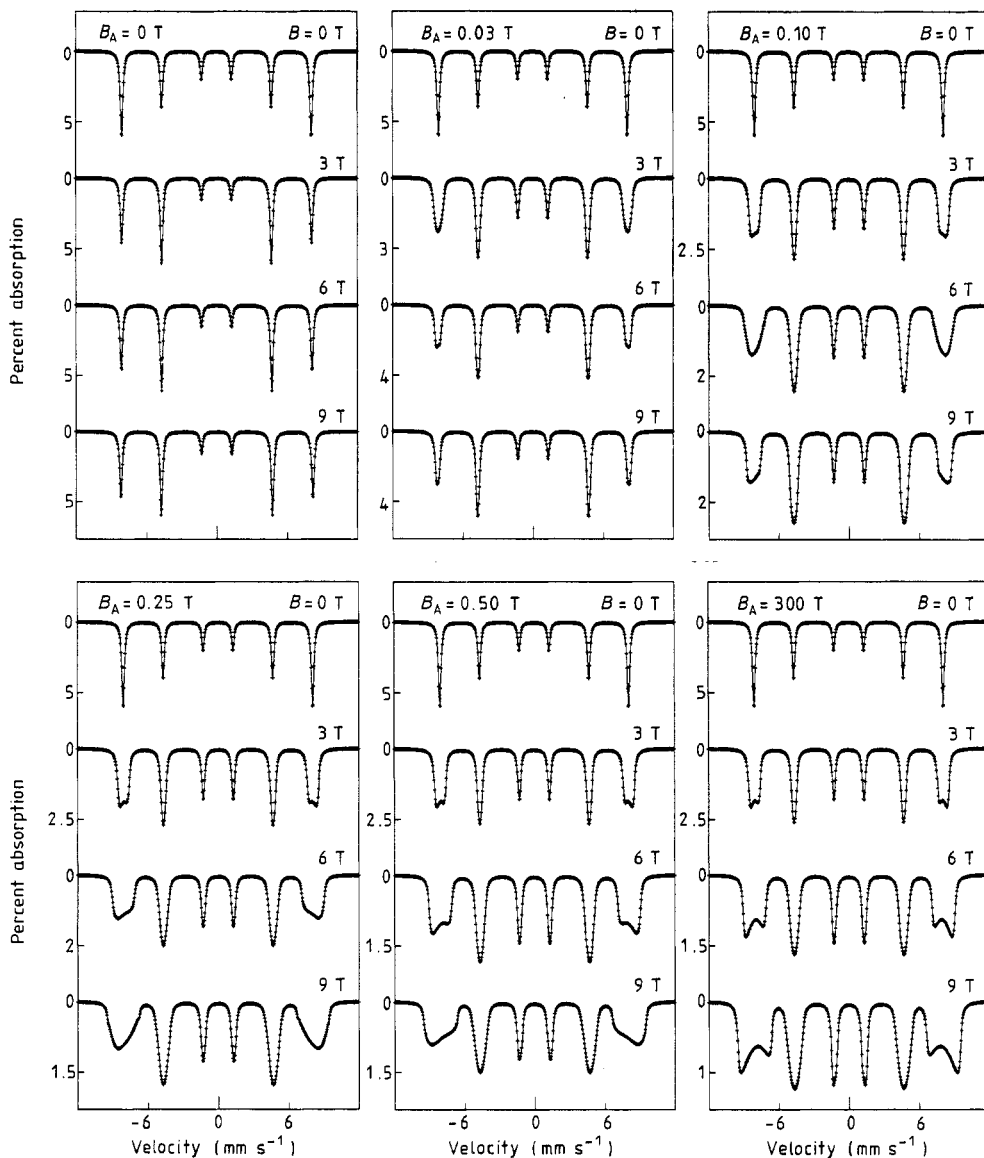
Figure 1. Simulated ^{57}\text{Fe} Mössbauer spectra of a powdered uniaxial antiferromagnet with hyperfine field B_{\text{hf}} = 50 T and exchange field B_{\text{E}} = 300 T subject to longitudinal magnetic fields of strength B = 0, 3, 6 and 9 T. Sets of spectra are shown for anisotropy fields B_{\text{A}} = 0, 0.03, 0.10, 0.25, 0.50 and 300 T.
